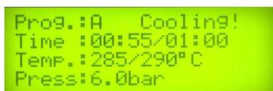
After the cooling mode, the piston will go down and the machine beeps three times.
