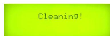
After automatic cleaning, the program will automatically go back to the Starting mode/ Idle mode, Clause 5.2.
